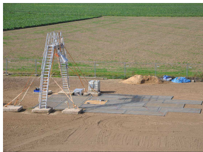
Figure 1. View of the experimental setup with the radiometer fixed on an arc and the sand box in the middle of the mesh grid at the TERENO test site Selhausen (Germany).
