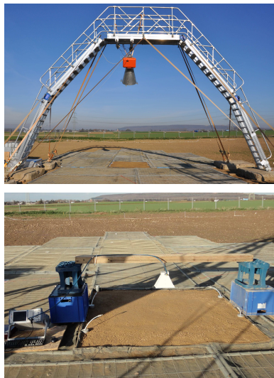
Figure 3. L-band radiometer ELBARA II mounted on the arc (top) and off-ground GPR antenna fixed above the sand box (bottom).
