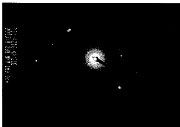
Fig. 17: A selected area electron beam diffraction pattern of Z phase.
