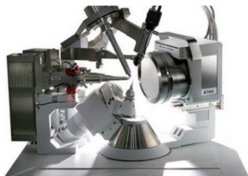
Abbildung 3.5: The OxfordDiffraction SupraNova diffractometer.
