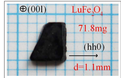
Abbildung 3.17: The \text{LuFe}_2\text{O}_4 single crystal used for neutron experiments in this and other work [1].
