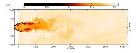
Figure 6. Instantaneous image of CO2 mass fraction from the LES of the IFRF furnace.
