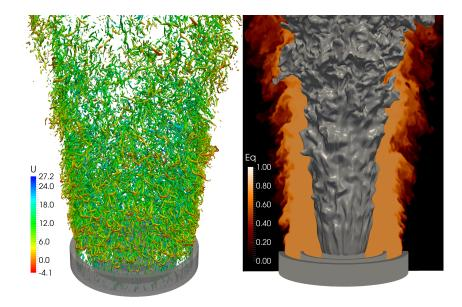
Figure 3. Left: Turbulent structures visualised by the Iso-q-criterion. The colouring corresponds to the axial velocity component (U / (m/s)). Right: Contours of equivalence ratio in the mid-section of the burner. The isosurface for 50% of reaction progress gives the flame location.
