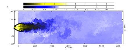
Figure 5. Instantaneous image of volatile gas mixture fraction (yellow scale) and char-off gas mixture fraction (blue scale) from the LES of the IFRF furnace.
