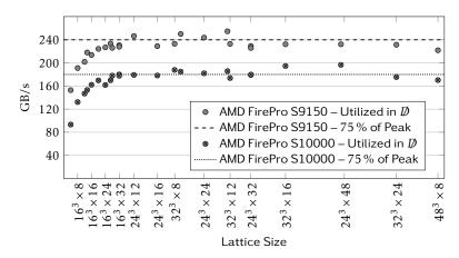
Figure 4. Benchmark of *D* for the L-CSC GPUs (taken from Ref. 14).
