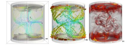
Figure 2. DNS data: (Left) configuration of the cubic computational domain showing the rotating impellers and the flow confining cylinder. (Middle) temporally averaged velocity profile. (Right) snapshot of volume rendering of the of the turbulent vorticity.
