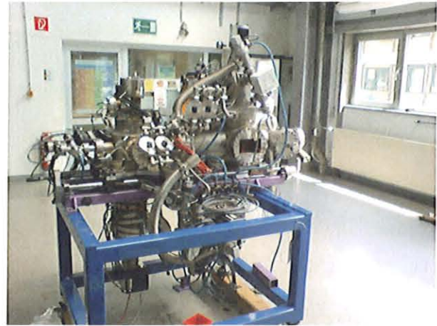
Fig. 22: The reassembled Breit-Rabi polarimeter on the new support.
