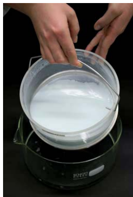
Figure 10-4 Batch binding cell containing \text{Ni}^{2+} -IDA sepharose for the purification of the fusion proteins DsbA/EK L and DsbA-EK-H6.
