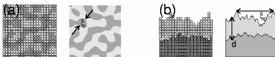
Figure 5.1: Sketch of systems with relevant mesoscopic or macroscopic properties. (a) Ferromagnet close to the Curie temperature. Ordered regions with a correlation length \xi exist. (b) Monolayer system. The layer thickness d and the in-plane correlation length of the rough surface \xi_p are much larger than the atomic spacing. The left picture of each example shows the real atomic structure the right part the approximation as a continuous system.
