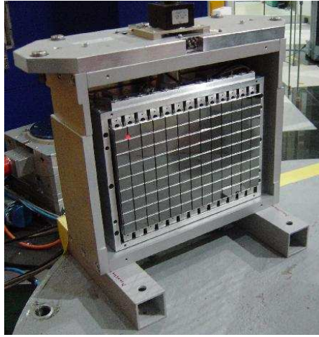
Figure 9.2: Pyrolytic graphite PG(002) monochromator of PUMA, the Göttingen-München thermal triple-axis-spectrometer at FRM-II.
