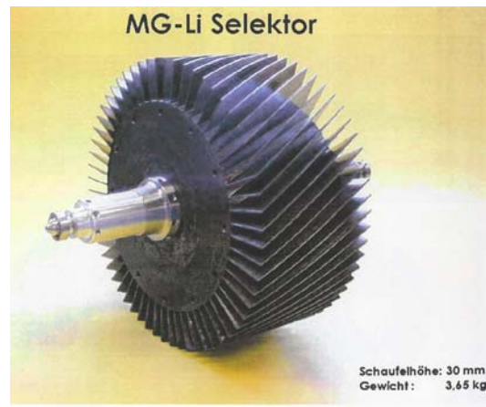
Figure 8.13: The rotor of the velocity selector of KWS-3 built at the FZ-Jülich.
