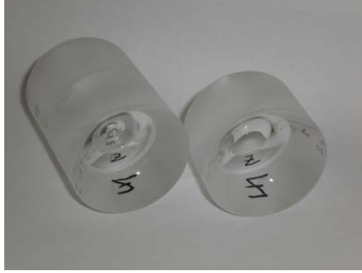
Figure 8.5: Aspherical \text{MgF}_2 lenses as focusing neutron device. The lenses are concave since the refractive index is smaller than unity for the neutrons. The lenses have a parabolic shape in order to reduce the spherical aberrations.
