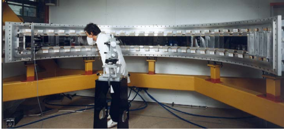
Fig. 8. Large 1600 element microstrip detector of the powder diffractometer D20 at the ILL Grenoble (F)
