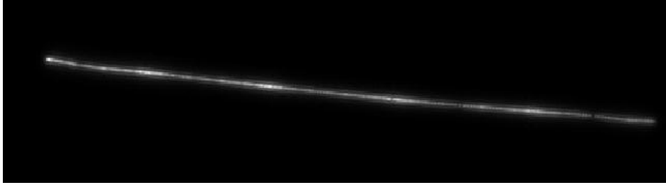
Figure 4.8: Image of the movement of the laser beam in the back focal plane. Images for 340 different motor positions were added, starting from the center position of the angle to positions where no fluorescent signal is normally detected in TIRF microscopy. The variation of the angle was not simply in one direction, but an overlap of x and y movement. The reoccurring brighter parts of the image represent areas, where the angle changed less rapidly, probably due to mechanical properties inside the TIRF-slider.
