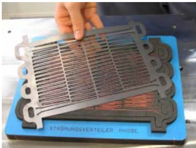
Fig. 25: Flow structure manufactured by die-cutting
