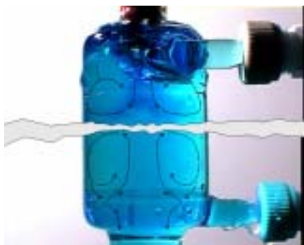
Fig. 61: Turbulent flow field in the glass model of an autothermal reformer: visualized using coloured water for the introduction of a steam flow (top) and an air flow (bottom)
