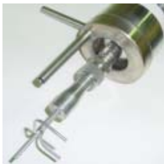
Fig. 67: Mixing chamber – upper section of the ATR-8 reactor with cooled nozzle fitting
