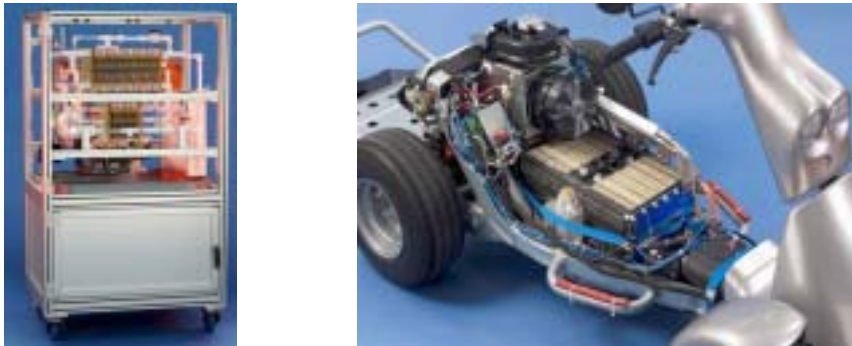
Fig. 51: 2 kW DMFC module from 2003 (left) and DMFC fuel cell system in an electric vehicle (scooter) from 2005 (right)
