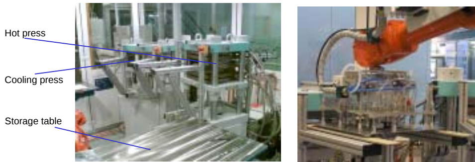
Fig. 20: Automated pressing system for MEAs (left); robot grapple system (right)
