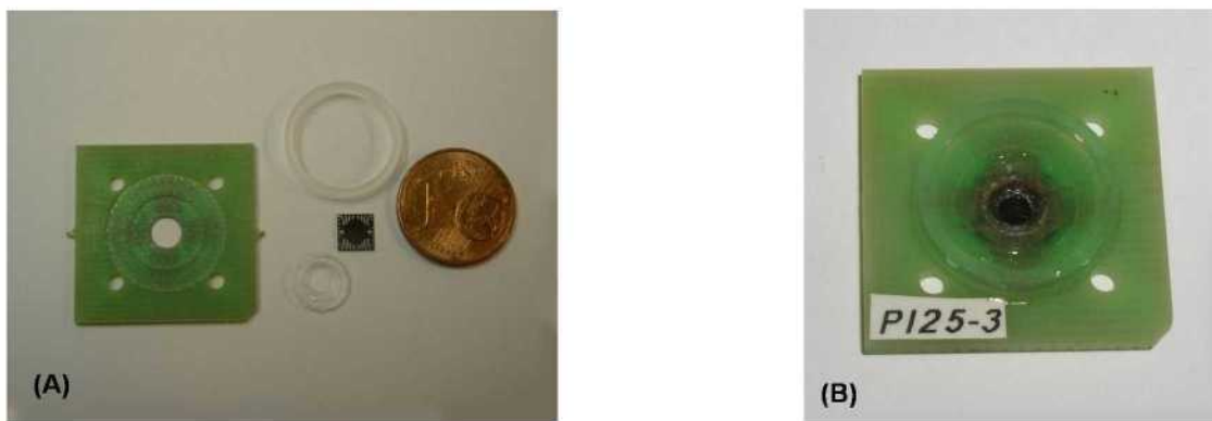
Figure B.3: The single components (A) were assembled to a chip holding a small petri dish on top (B).
