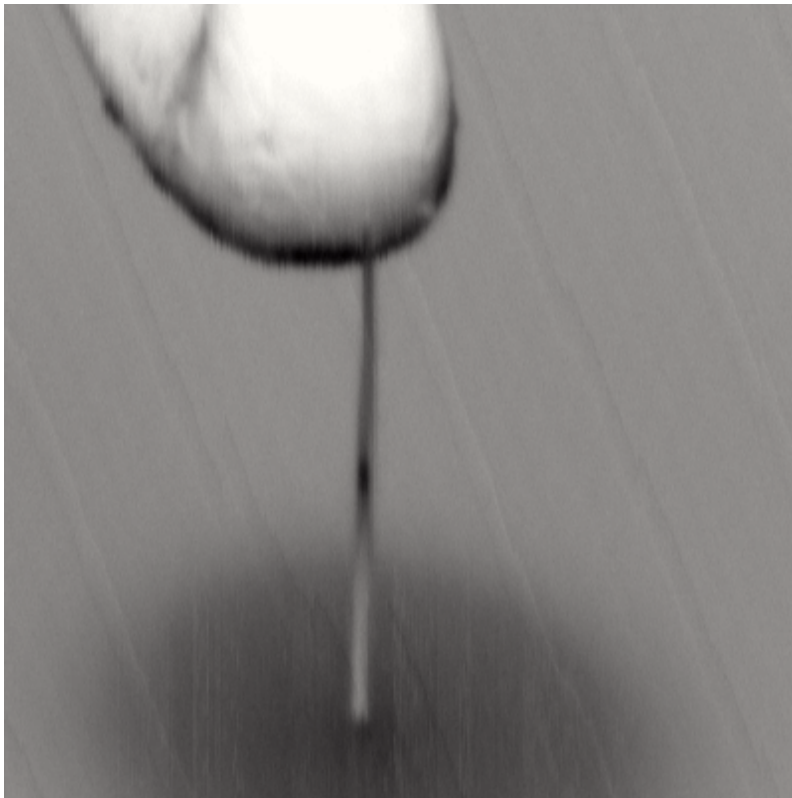
Figure 6.2: SEM image of the long run measurement configuration. A nanowire is contacted by a single STM tip. The picture was taken using the current flowing through the sample for contrast.
