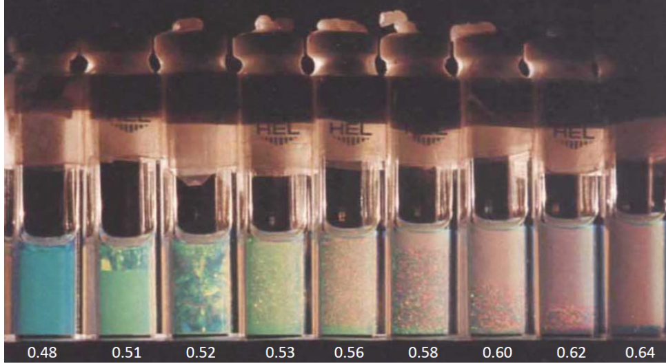
Fig. 3: PMMA particles suspended in an refractive index matching solvent mixture at effective volume fractions indicated by the numbers at the bottom. The samples are illuminated obliquely from behind with white light. Homogeneous colors indicate a random distribution of particles while opacity is due to Bragg diffraction, indicating crystal structures with lattice constants in the wave length range of visible light. Image reproduced from reference [45] with permission.
