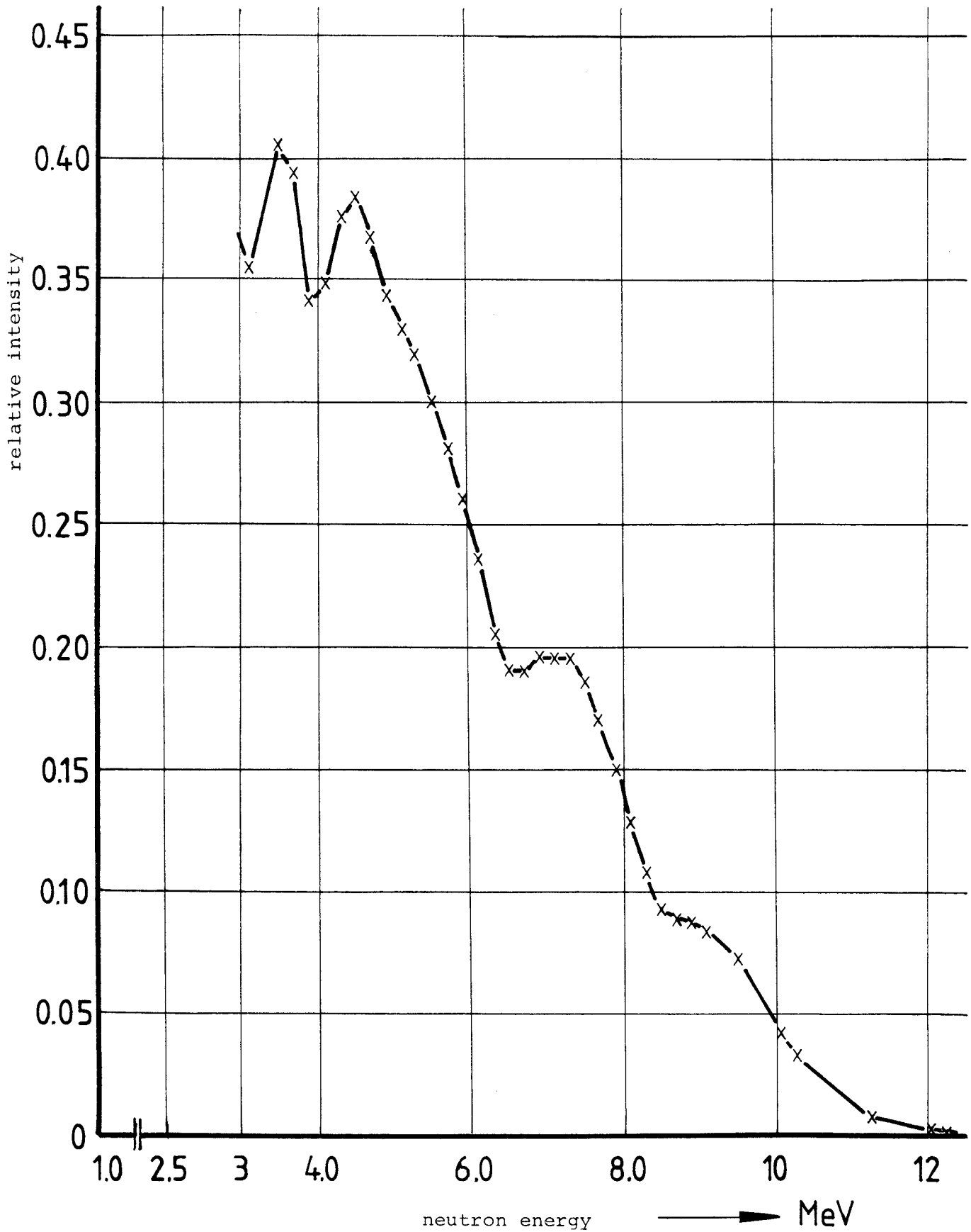
Fig. 5.4: The first iteration neutron spectrum of Am-Be neutron source with the 2"x5" NE-213 scintillator
