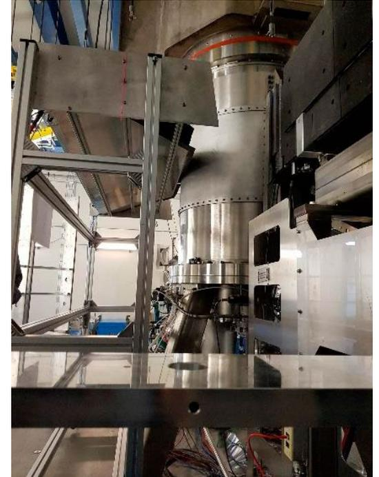
Mantle detector mounting unit touching POWGEN detector vessel (aus arXiv:2110.12767)
