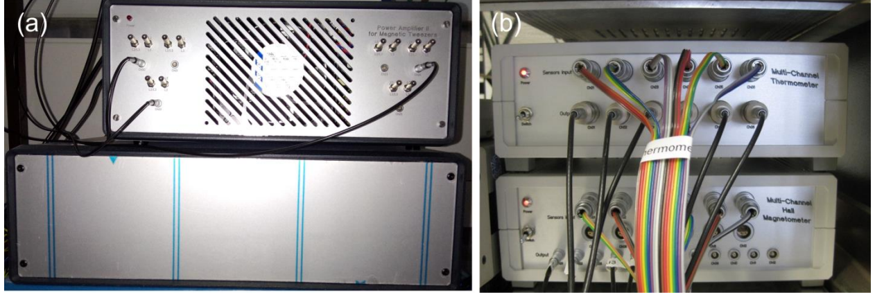
Fig. 3.4. (a) The power amplifier II. Top: amplifier, bottom: bipolar DC power supply. (b) Thermometer and magnetometer.
