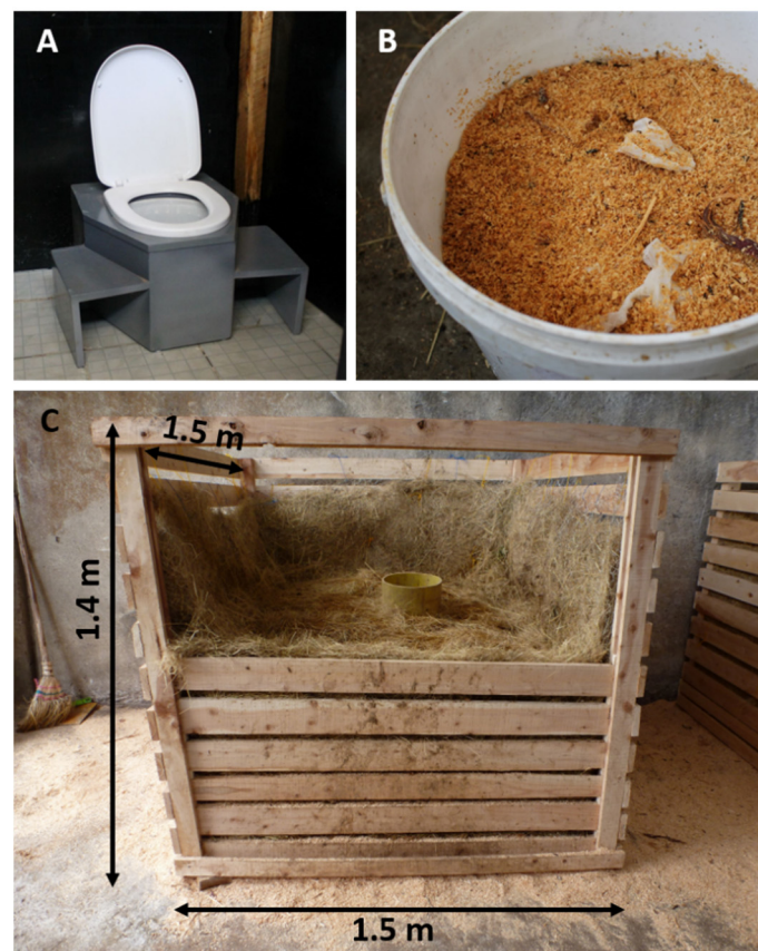
Figure 1. An installed dry toilet (A); a toilet bucket filled with collected materials (B); and a compost box after experimental set-up with dimensions (C) (Photos: K. Prost and K. A. Werner).
