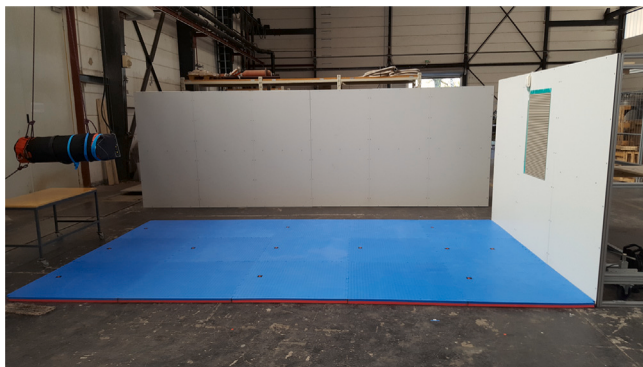
Fig. 1. The experimental area covered with mats has a size of 3 m × 5 m. On the left side, a punching bag was suspended from the ceiling to push the participants forward. The right side of the area was limited by a solid wall.
