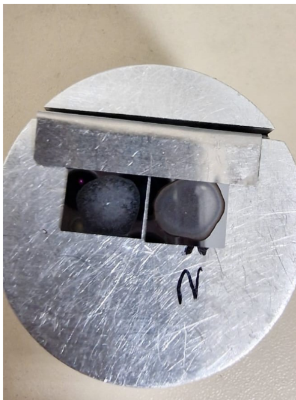
Figure 22: SEM holder with fungus sample. The right sample is for the fungus with \text{AgNO}_3 NPs and the right sample is for funges without \text{AgNO}_3 NPs.
