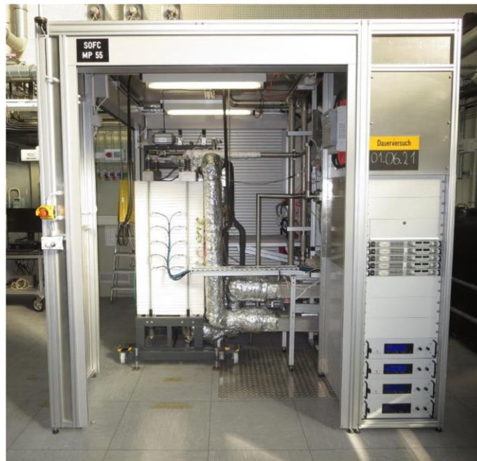
Figure 3. Test environment of the system in the laboratory. The white rectangular block the center of the picture is the thermally insulated Integrated Module.
