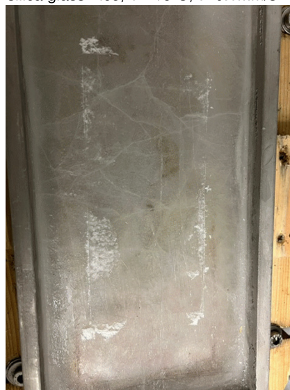
FIG. 16. Ice surface after sliding in Fig. 15. Note the ice wear particles (white powder).
