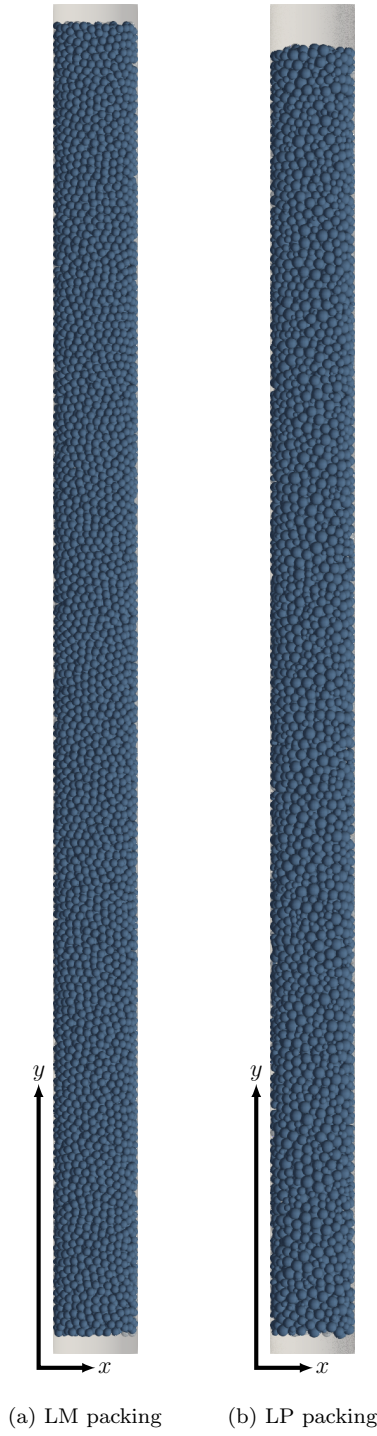
Figure 8: Geometry of long mono-disperse (LM) and long poly-disperse (LP) packings.
