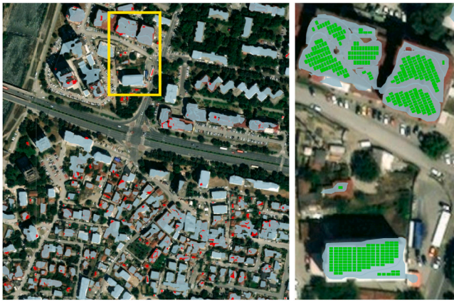
Fig. 11. District of Skopje, North Macedonia analyzed in Adjiski et al. [60]. The GUI visualizes the final sections in blue, with the sections filtered by size in red and panels in green. The buildings used for the final analysis are zoomed on the right. The background map corresponds to Bing Maps imagery. (For interpretation of the references to color in this figure legend, the reader is referred to the web version of this article.)
