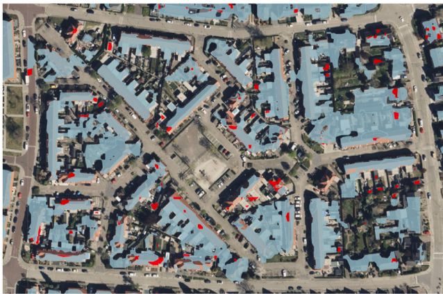
Fig. 12. A picture of the district in Apeldoorn, the Netherlands that was used in the figures of Kausika et al. [61], and the results of PASSION. Sections that were filtered due to their size are shown in red, and those that were used in the study appear in blue. The background map correspond to Bing Maps imagery. (For interpretation of the references to color in this figure legend, the reader is referred to the web version of this article.)
