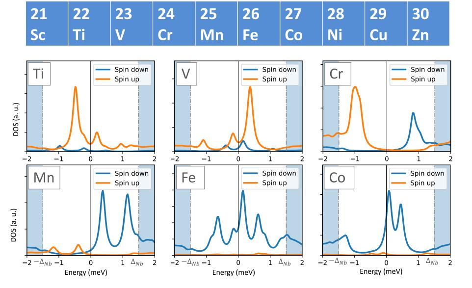
Specific YSR states patterns arise from the different magnetic impurities, depending on the orbital's interactions with the Nb crystal field.
