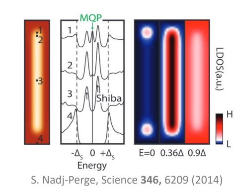
At some given chain length, the quasiparticle interferences trapped inside the chain create a zero bias peak located at the chain's ends. This state is topologically protected by the superconducting gap, providing robustness suitable for creating fault-tolerant qubits.
