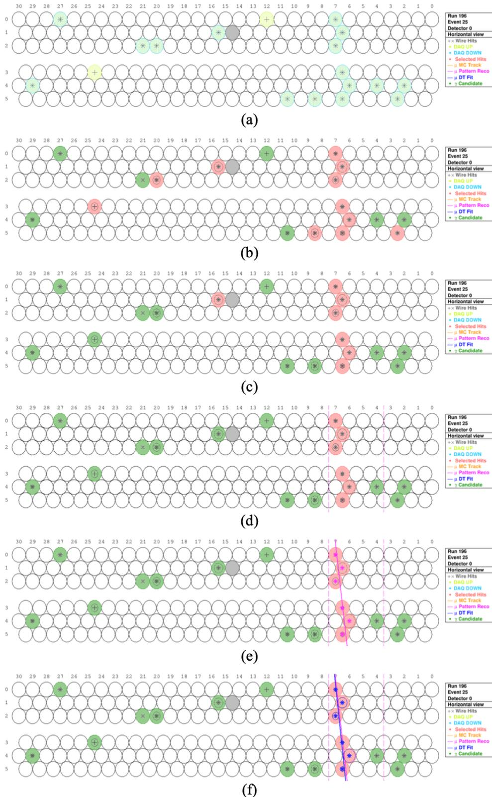
**Figure 6** (a) Hit collection of one event recorded during MUTOMCA field test, in presence of a cask with three dummy bars. (b) Effect of the time filter. (c) Effect of the space filter. The filter does not apply to the tubes close to a dead channel (in grey) in order to avoid further inefficiencies in that area. (d) Area selected by the clustering algorithm. (e) Track candidate find by Pattern Recognition step. (f) Drift Time fit.
