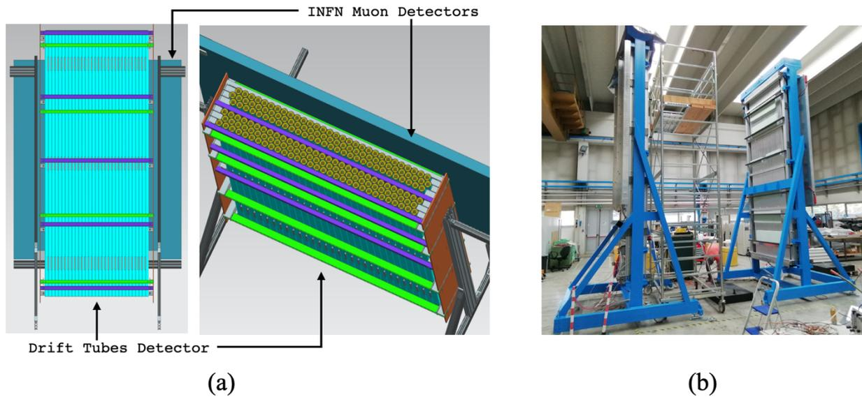
**Figure 1** (a) Design of one detector module developed for the MUTOMCA project. (b) A picture of the complete muon detector assembled in Laboratori Nazionali di Legnaro.
