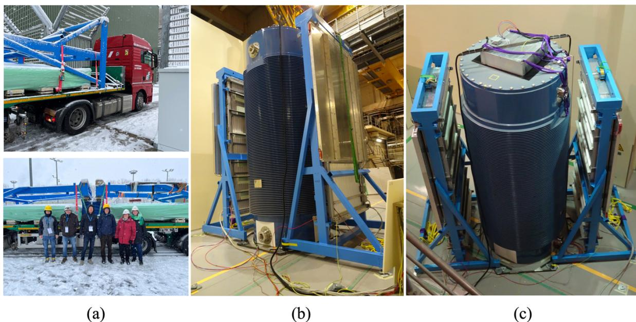
**Figure 5** (a) Pictures of the detector arrival at the SFSF site of Grafenrheinfeld, January 18<sup>th</sup> 2023. (b) Picture of the experimental setup during data-taking. (c) Experimental apparatus seen from above: the small drift chamber used for alignment purposes is visible on the top of the cask.
