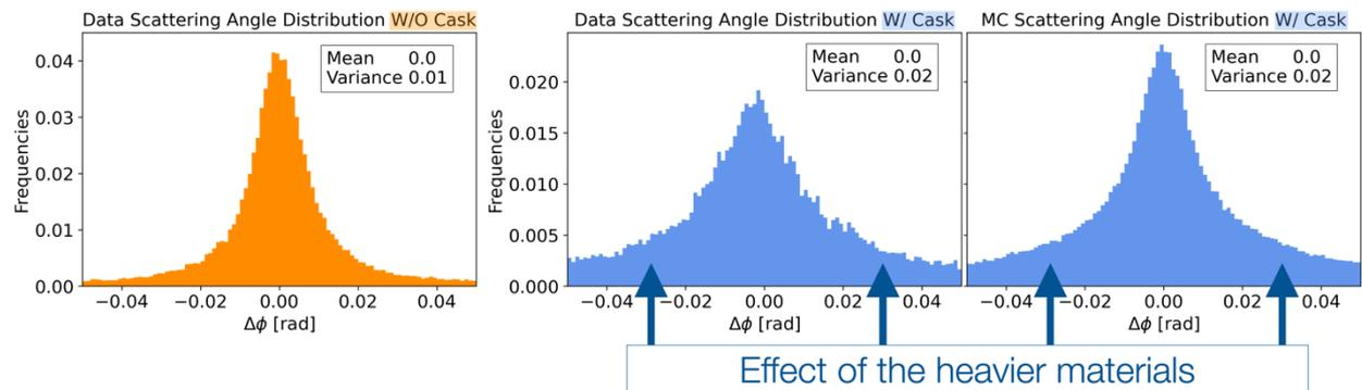
**Figure 7** From left to right, distribution of the scattering angle in data without cask, in data with cask and in MC simulations with cask.
