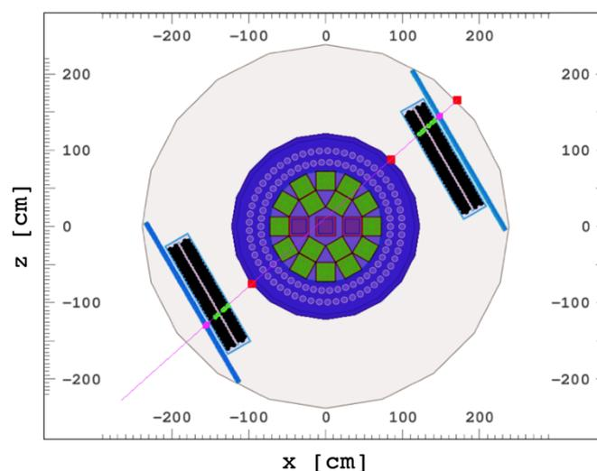
**Figure 3** A display of one event generated with the MUTOMCA Monte Carlo simulator. The simulated CASTOR V/19<sup>®</sup> contains three dummy elements in the center.
