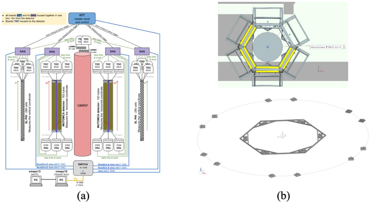
**Figure 2** (a) Scheme of the electronics of the MUTOMCA experimental setup. (b) Scheme of the detector positions in the test location and system of support pads for precise positioning.
