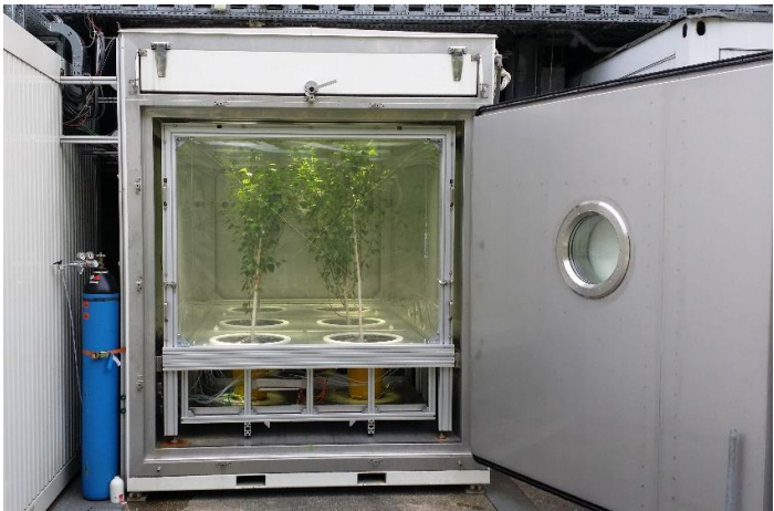
Figure 2-8. Sweet chestnut trees were placed inside the SAPHIR-PLUS chamber.
