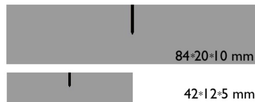
Figure 7. Sketch including pre-notch and dimensions for both the large and the medium-sized samples.
