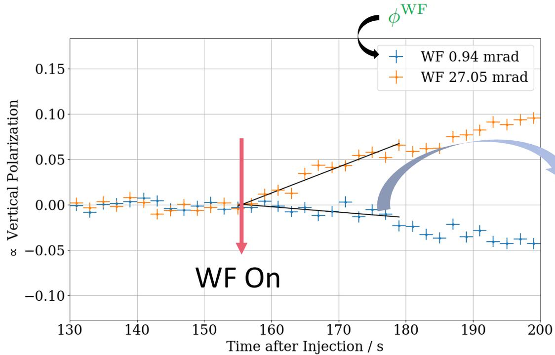
$$\epsilon^2(\phi^{WF}) \propto |\vec{n}_{WF} \times \vec{n}|^2 \quad \vec{n}_{WF} : B \text{ field axis of rf Wien filter} \quad \vec{n} : \text{ISA}$$
