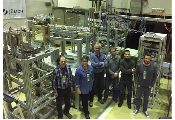
Fig. 49: Installation of the test systems in the former COSY-TOF beam area. The beam enters from the back.
