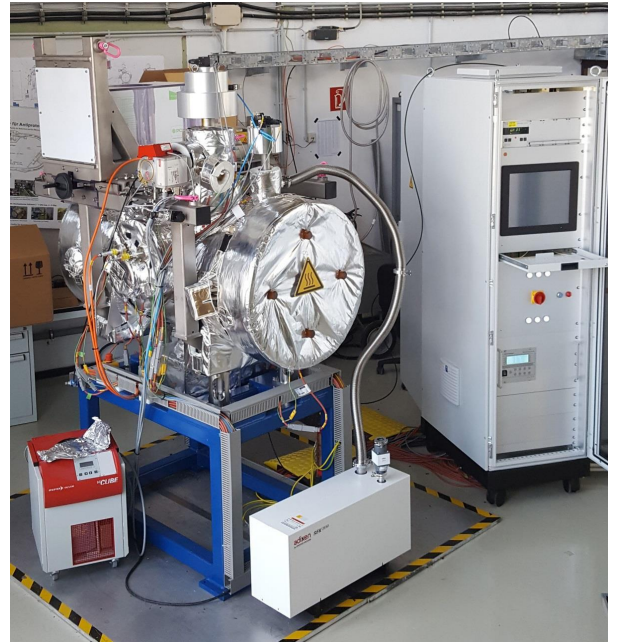
Fig. 33: Photo of the injection kicker test tank with lifting mechanism, protective covers, heating jackets, pumps, and control rack. It will be used to determine the stray capacitances and stray inductances with the magnet installed.
