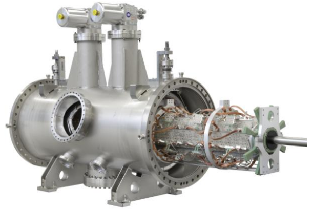
Fig. 39: Stochastic cooling chamber (pick-up) before final installation in the clean room.
