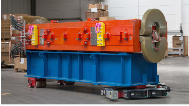
Fig. 32: Complete HESR dipole magnet being moved to the final storage place inside the storage hall in Darmstadt. Motor driven wheels allow a denser packing than using conventional trolleys.
