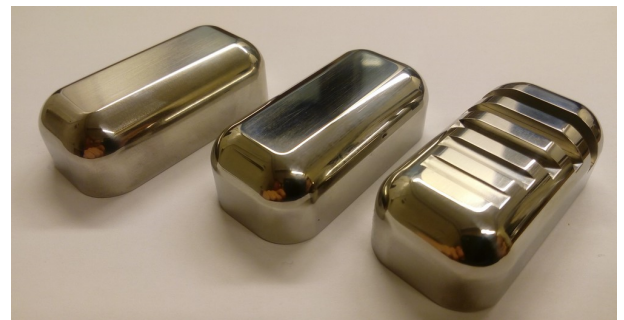
Fig. 24: New electrodes for testing field-measurement technique.
