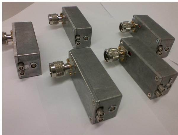
Fig. 3: A photograph of the HESR BPM preamplifier prototypes.
