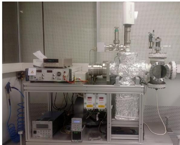
Fig. 1: The test bench for electrostatic deflectors.
