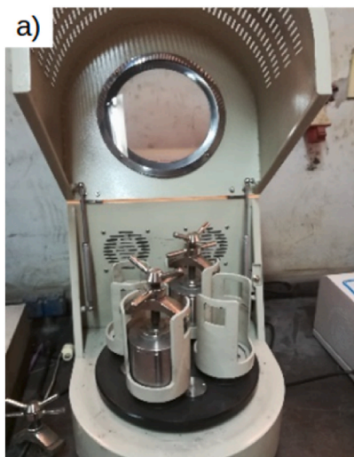
Fig. 2. (a) The planetary ball milling machine used for powder mixing and milling, and (b) a schematic representation of the ball milling process. CW and CCW stand for clockwise and counterclockwise directions, respectively.
