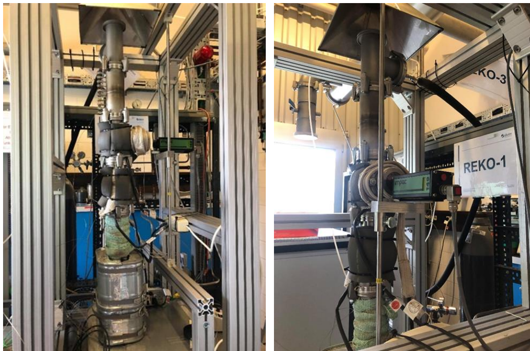
Figure 2. REKO-1: Cylindrical flow reactor (left); catalyst temperature measurement (right) [8].
