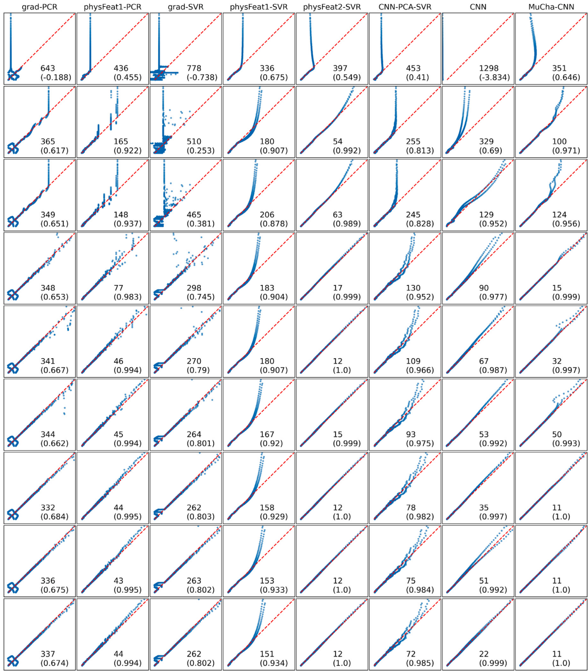
Fig. C.17. Confusion matrix of all models for training with different sizes of the Cahn–Hilliard dataset. The vertical and horizontal data ranges (energies) for each sub-plot are 0..8000. The number inside the sub-plot represents the RMSE value (without brackets) and R^2 score (with brackets).
