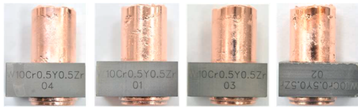
Fig. 7. W-10Cr-0.5Y-0.5Zr blocks after OFHC-Cu casting.
