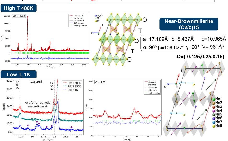
**LSMO powder, INTER. 2 (more V**<sub>0</sub>), Vibrating Sample Magnetometer(PPMS-VSM)
