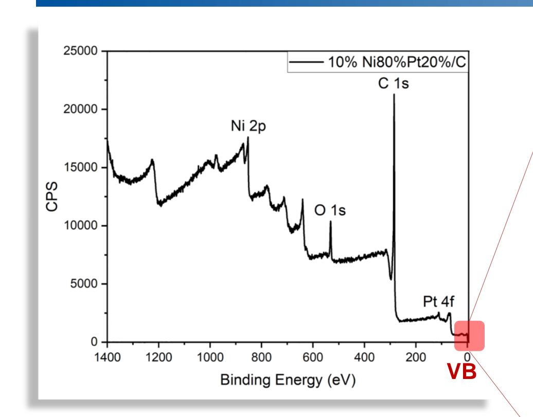
Monochromatized Al kα XPS survey Spectra of 10% weight loading on Ni80%Pt20%/C reduced (H<sub>2</sub> flow for 1 h at 250°) catalyst
