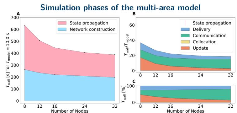
Strong-scaling benchmark of macaque multi-area model performed with NEST v3.6 on Jülich Supercomputer JURECA.
