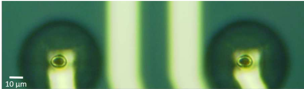
Fig. 39: Light microscopy image of hollow cylinders printed with low degree of polymerization and thus leading to structural deformation.
