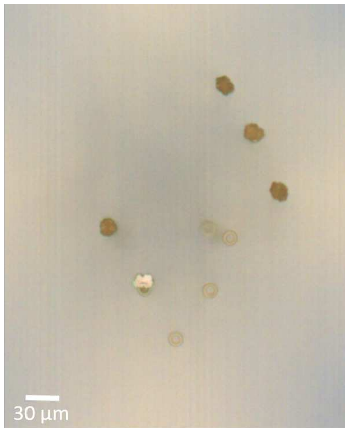
Fig. 60: Light microscopy image of printed cylinders with 150\ \mu\text{m} height. Applying -200\ \text{nA} for 1\ \text{min} leads to gold caps of around 20\ \mu\text{m} diameter.
