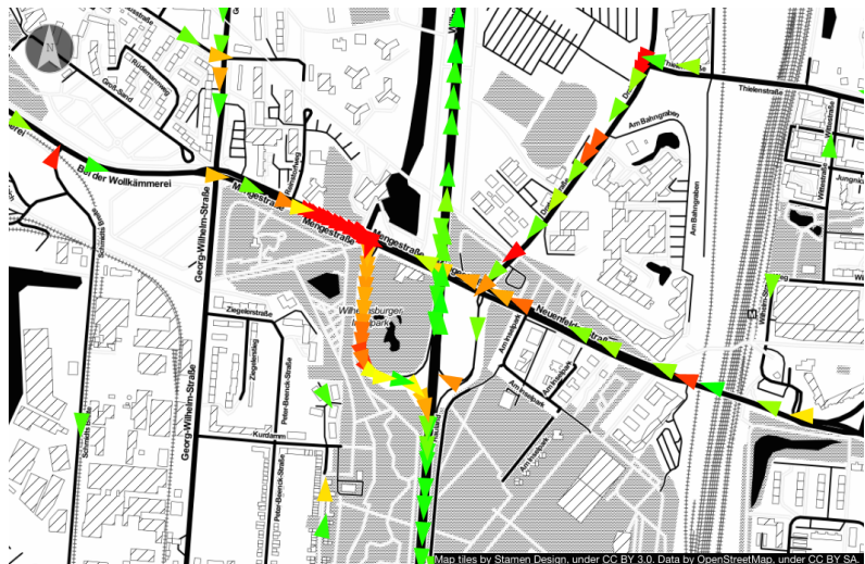
Figure 8. Situation about 20 minutes into simulation showing vehicles in congestion (indicated by the nongreen triangles) at and around an on-ramp to the Wilhelmsburger Reichsstraße, one of the major evacuation routes.
