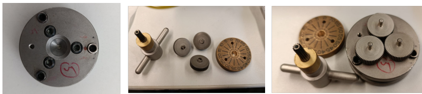
Figure 5.17: Boehler-Almax Diamond Anvil Cell is made from stainless steel with a screw drive to apply pressures.
