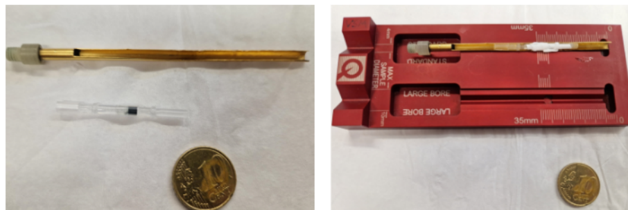
Figure 5.4: (Left) Sample filled into a VSM plastic capsule. (Right) The plastic capsule covered with Teflon is loaded into the brass sample holder in preparation for the VSM measurement.
