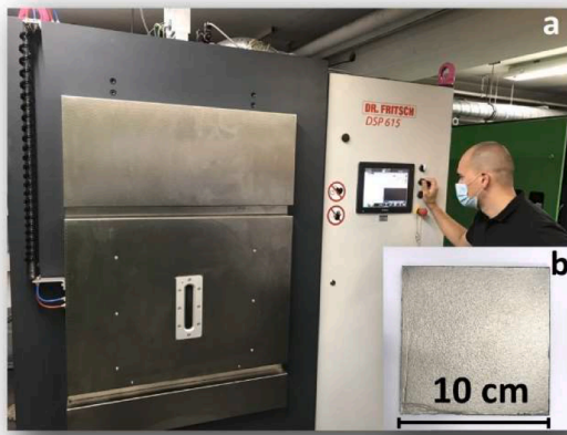
Fig. 3. Field-assisted sintering technology of SMART materials at industrial scale: a) sintering of SMART sample in DSP 615 facility at Dr. Fritsch GmbH from the powder produced by Zoz GmbH and b) the rectangular SMART sample produced at FZJ, using the industrial FAST facility Dr. Fritsch DSP 515 using know-how of Dr. Fritsch, powder from Zoz GmbH, programming from FZJ. The sample features a relative density which exceeds 97 %.
