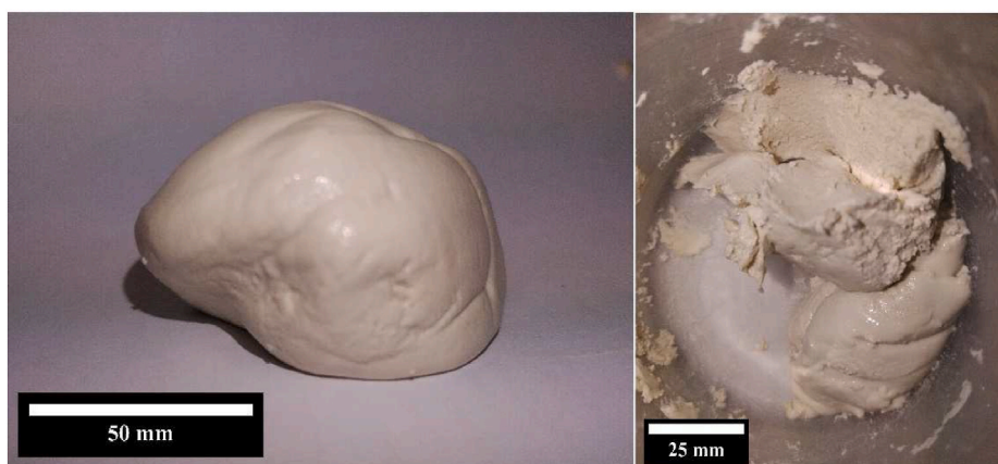
Fig. 11. ASH-G samples 2, 3 and 4 behaved more as a solid than a liquid (left). Instead of flowing, samples would tear upon mixing with a high shear impeller (right).
