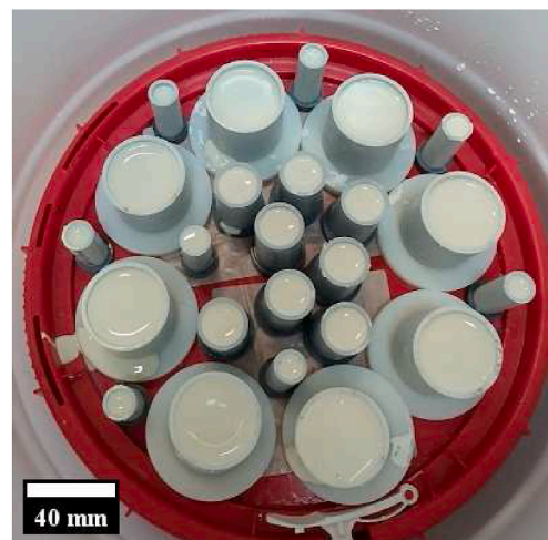
Fig. 1. Wet ASH-G in cylindrical molds before curing for 7 days. Only the largest cylinders were used.
