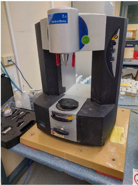
Fig. 4. Kinexus Pro + rheometer used to measure yield stress and viscosity. The bottom and top plates are not included in this photo.
