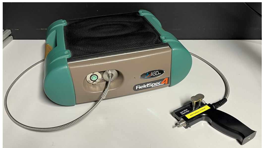
Figure 3. Example device: ASD FieldSpec 4 Standard-Res portable spectroradiometer.
