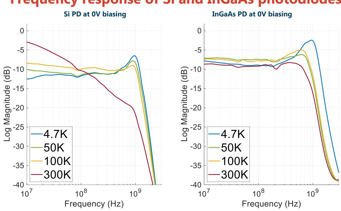
Both photodiodes shows higher bandwidth in cryogenics due to the decrease in junction capacitance with temperature
