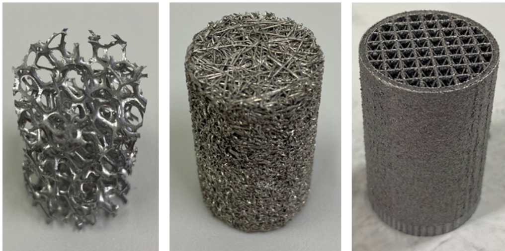
Figure 4.20: Different samples of porous structures made of aluminium. Aluminium foam (Fraunhofer IWU, left), sintered fibres (Fraunhofer IFAM, center) and an additively manufactured grid (Forschungszentrum Jülich, ZEA-1, right)
