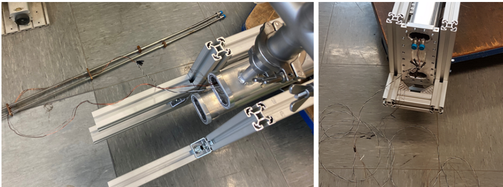
Figure 5.8: Assembly of the transfer lines into the vacuum recipient with attached sensors and heater cable.
