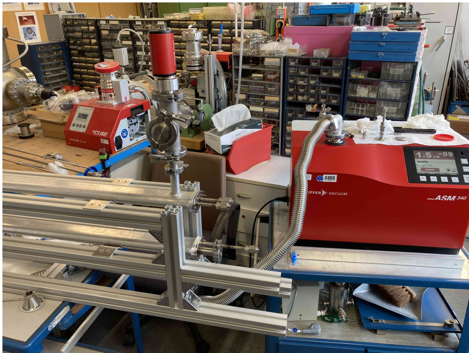
Figure 5.12: Helium leak test of the vacuum recipient using a mass spectrometer.
