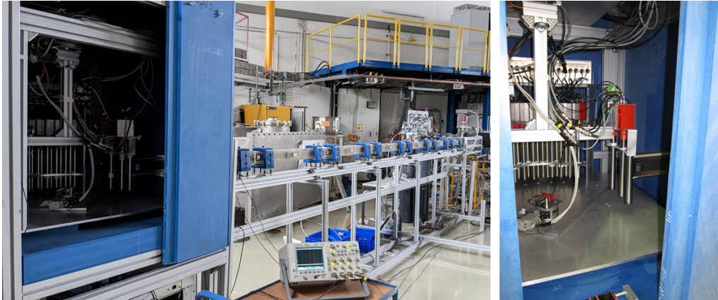
Figure 6.7: Opened detector assembly box (left side of left photograph) shielded by walls of borated polyethylene (blue) and including multiple ^3\text{He} detector tubes (right).
