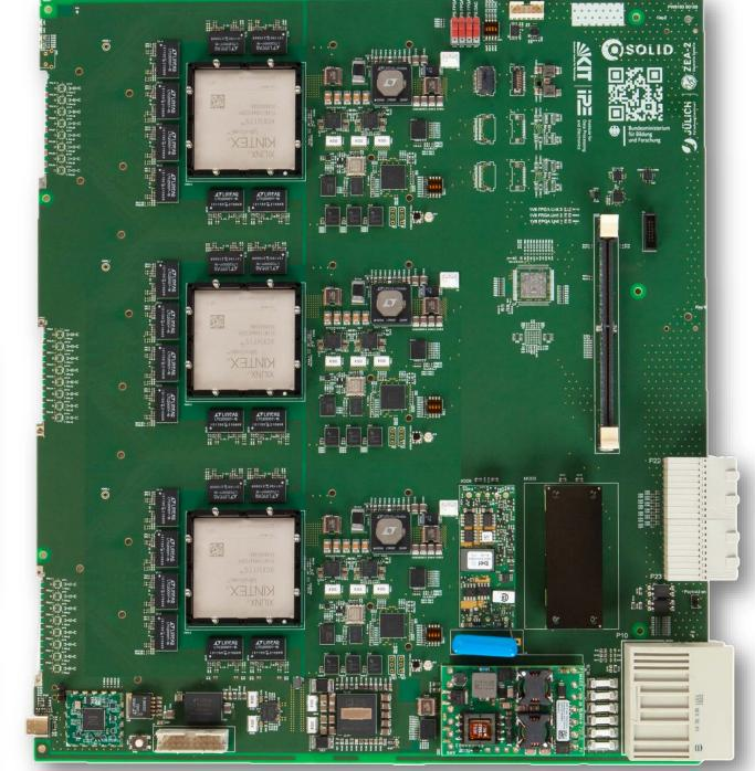
The **Hub** card (illustration) consists of the **iW Rainbow G42M** SoM with an AMD ZU49DR **XCKU115** with eight RFSoC allow software defined qubit readout and control to the required center frequency between 4-7 GHz and a channel spacing of 50 MHz. Controls up to 10 interconnected FPGAs through the backplane of the **ATCA** crate [1,2].
