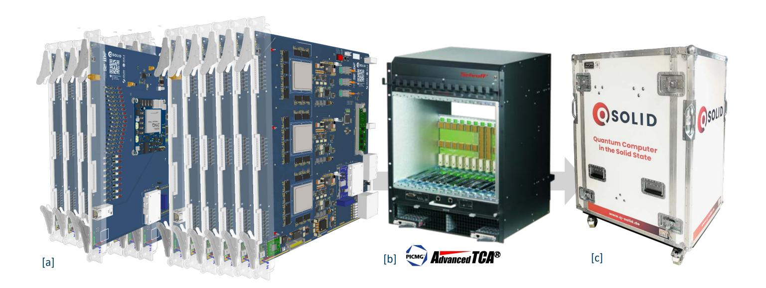
a) Illustration of a full assembled ATCA crate insert. Holding 4 Hub cards capable of reading and controlling 40 qubits, mastering up to ten additional Node cards capable of driving 24 direct flux lines each. b) Interconnectivity, thermal management and power through Dual-Dual-Star crate from nVent Schroff, based on PICMG standard AdvancedTCA [1,3]. c) Shock protection transportation box from ProCase.
