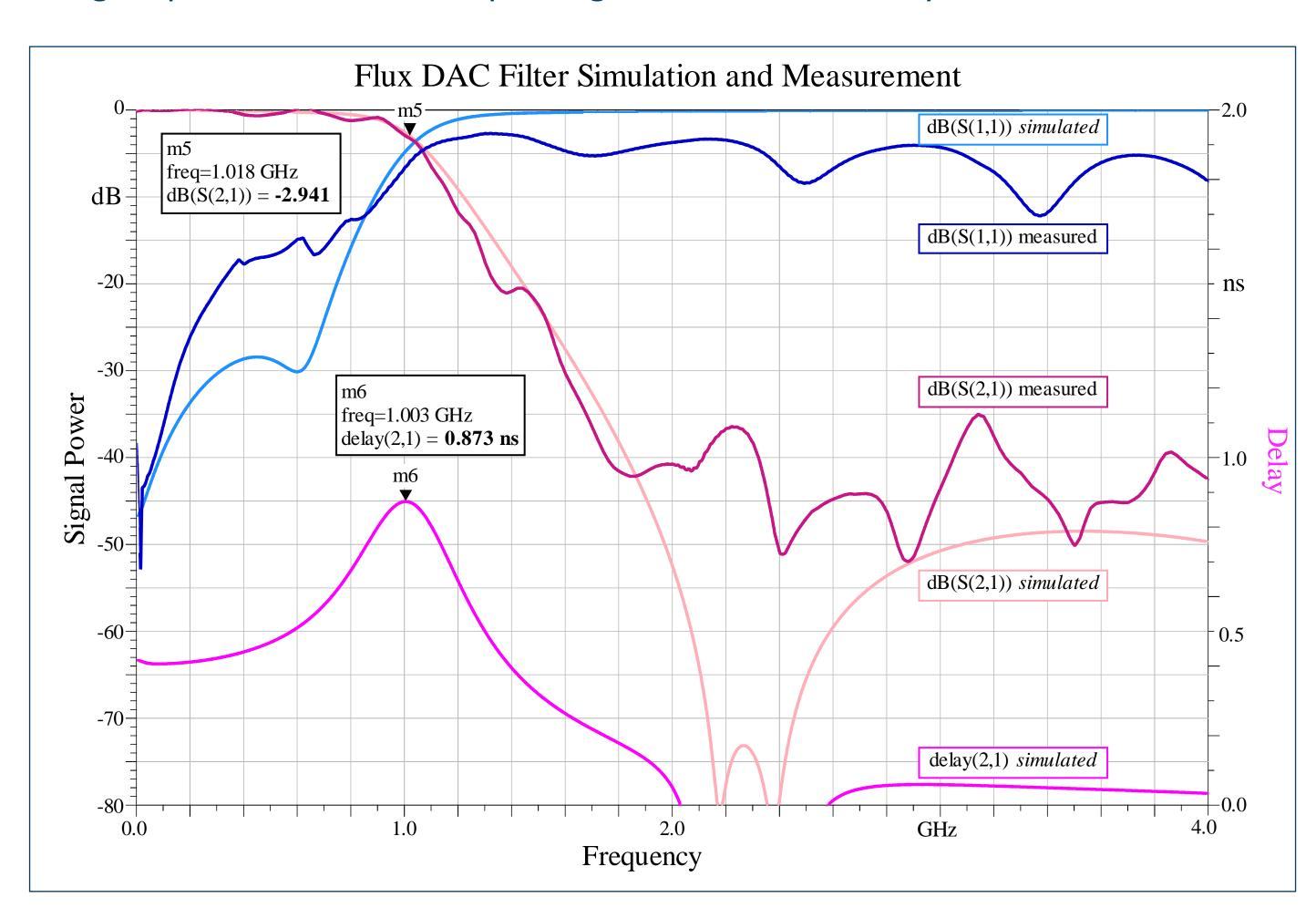
Flux signal output from **DC to 1 GHz @ 10 dBm,** tunable to a cutoff frequency from 0.5 to 1 GHz with a **group delay** of **0.8 ns**. Filter specific notches in stopband suppress the digital DAC frequencies
