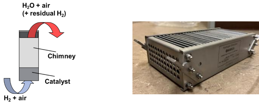
Fig. 1. (left) principle sketch of a recombiner; (right) commercial recombiner for battery rooms.
