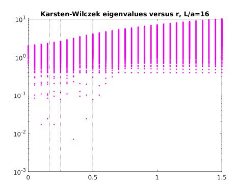
Spectrum at r = 0 is naive (i.e. 4-fold staggered) spectrum.
