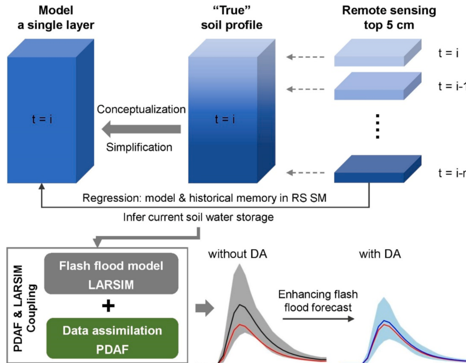
Fig. 2. Schematic of the framework for assimilating RS SM into flash flood simulations. It describes the concept of using current and multiple antecedent RS SM to infer the current total soil water storage and assimilating the total soil water storage in flash flood models.
