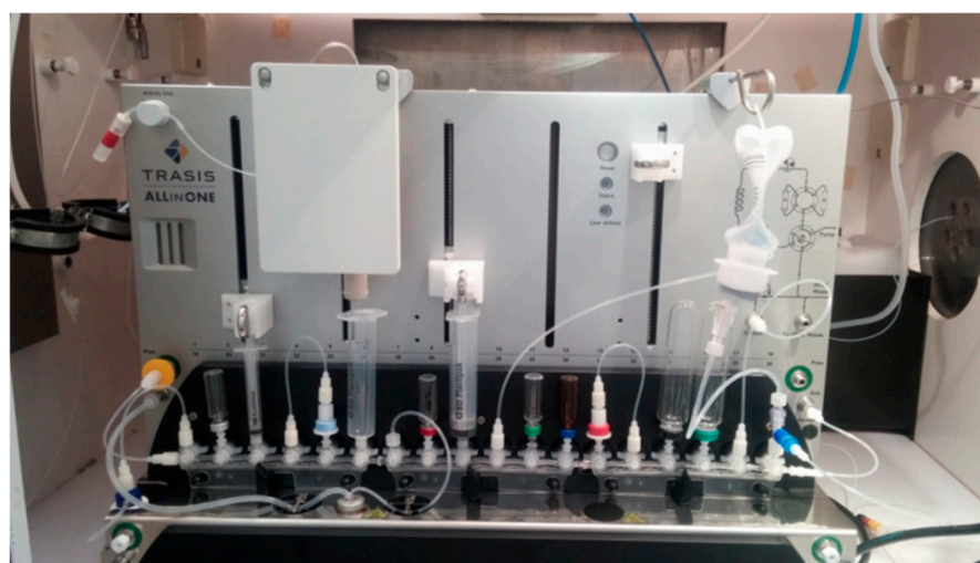
Figure 4. Trasis AllInOne synthesizer configured for the preparation of [ ^{18}\text{F} ]JK-PSMA-7.
